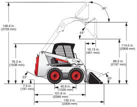
10 - 16.5 TIRES - 66.0" (1676 mm) or 60.0" (1524 mm) or 60.0" (1524 mm) 31.5 x 13 - 16.5 TIRES - 66.0" (1676 mm) "B" 10 - 16.5 TIRES - 54.5" (1385 mm) or 48.5" (1232 mm) 31.5 x 13 - 16.5 TIRES - 52.3" (1328 mm) 62 in. BUCKET WIDTH - 62.0" (1575 mm) 68 in. BUCKET WIDTH - 68.0" (1727 mm) 74 in. BUCKET WIDTH - 74.0 (1880 mm)
